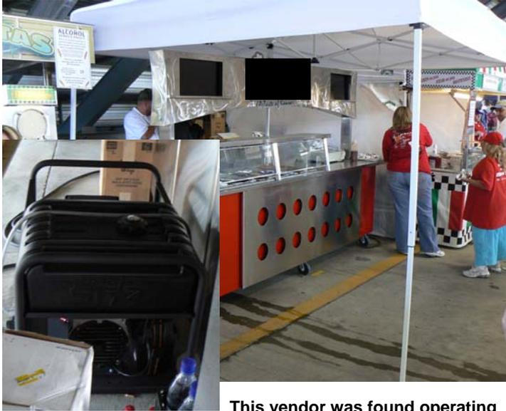
**This vendor was found operating a gasoline generator under a spectator seating area. The vendor was shutdown and the generator removed.**
